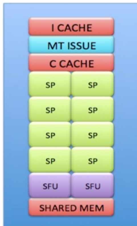
Figure 3.4 SM Multithreaded Processor (reproduced from [19])
